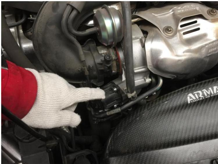
3. Remove the valve by disconnecting the plug and removing the 3 bolts.
