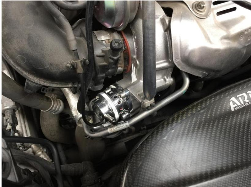
5. Locate the vacuum pump on the right hand end of the engine (when viewed from the front), and remove the small bore vacuum hose from the side of the outlet. Use the supplied tee piece as shown below to connect to the pump outlet with a short length of vacuum hose, and then connect the coil of vacuum hose to one other side and run it over to the BOV neatly.
