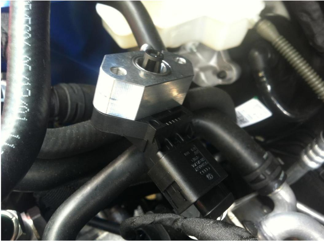
10. Fit the silicone vacuum hose to the alloy vacuum take off and dump valve.
