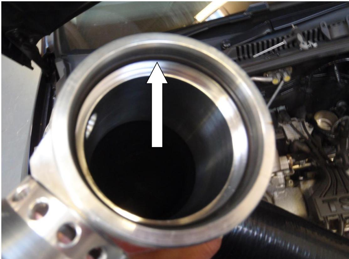
5. Fit the dump valve adaptor onto the inlet manifold making sure that the clips secure correctly.
