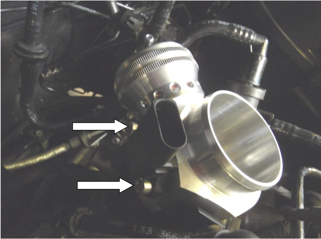
7. Fit the silicone hose using the supplied hose clips.
