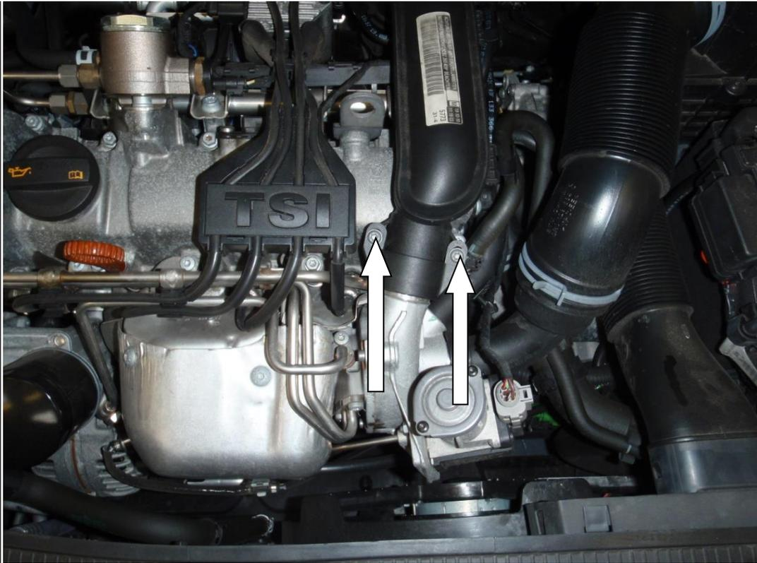
2. Remove the map sensor from the plastic boost pipe by removing the two T20 torx head screws.
