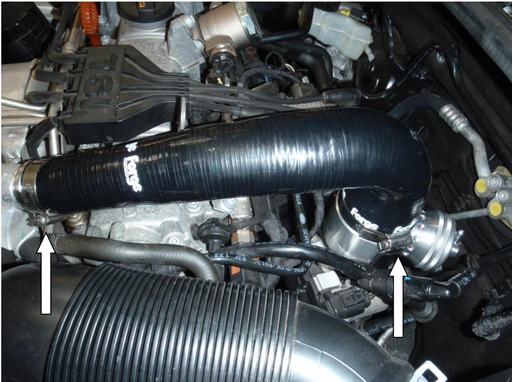
8. Unclip the second map sensor from the inlet manifold and insert the alloy take off.
