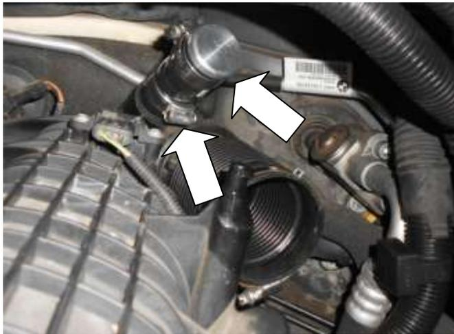
16. Place a suitable hose clamp over the small end of the silicone elbow and fit it to the standard pipe work.
