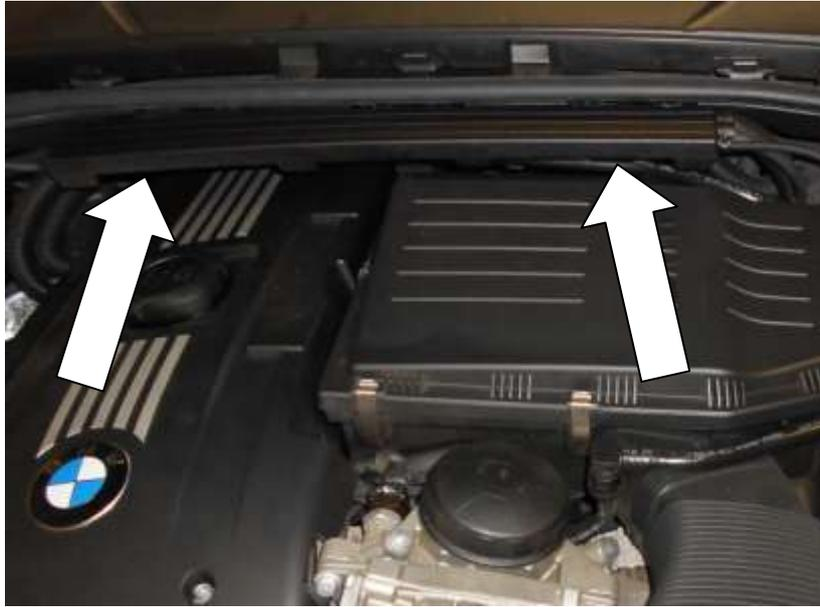
6. Using a short flat blade screwdriver undo both jubilee clips on the hoses either side of the air box. Slide the hoses off of their outlet.
