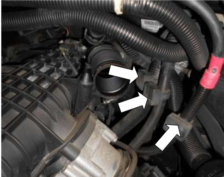
8. Twist the clip and pull off the pipe work running to both standard dump valves. Disconnect the vacuum hose running to the standard dump valves.
